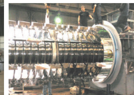
NVD-20-V5 (Segment Seal) [Wing outer diameter: 2000mm]
